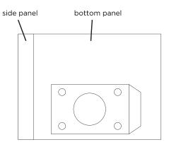
Attach the adjustable leg base with the flat side facing the outside of the cabinet.
