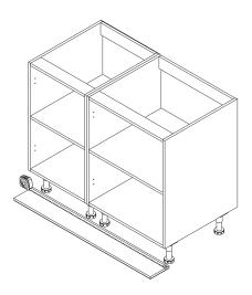
Draw a line 50mm front the top along the full length of the kickboard. Mark the centre of each adjustable leg on this line and then mark 16mm either side of this line. Attach kickboard clip.
