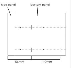
The adjustable legs that the kickboard returns attach too need to be moved in. Draw a straight line across the 2 predrilled holes and mark in from the side of the cabinet 56mm and 110mm on these lines.
