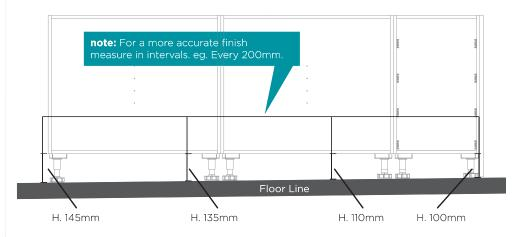
For uneven floors take the measurement from the floor to the bottom of the cabinet.
