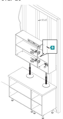
Check cabinets are level then clamp together. Pre-drill using 2mm drill bit and attach cabinets together.
