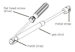
**note:** the gas strut can be adjusted by moving the bracket on the door forwards or backwards.
