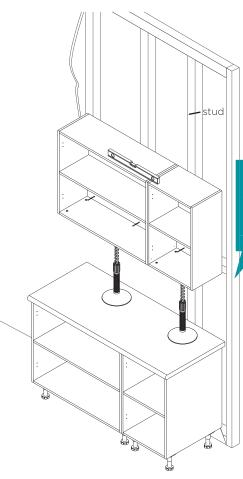
Caution: Please ensure all cabinets are screwed into your timber stud wall using a minimum of 65mm timber screws. If attaching to concrete, brick, steel or any other substrates seek advice from your hardware specialist.
