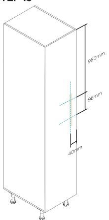
Place masking tape on both sides of the door where holes will be drilled to avoid chipping. Pre drill using 4.5mm drill bit
