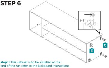
end of the run refer to the kickboard instructions now on the correct placement of the feet. Set the height of the adjustable feet to 145mm to suit the kickboard.
