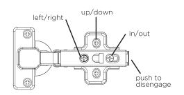
Clip the door onto the hinge plates.
