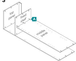
**note:** Make sure the shelf support holes on the middle panel face the support holes on the side panel.
