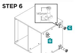
**stop:** If this cabinet is to be installed at the end of the run refer to the kickboard instructions now on the correct placement of the feet. Set the height of the adjustable feet to 145mm to suit the kickboard.
