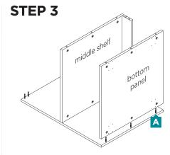
**note:** Make sure the pre-drilled holes for the adjustable feet are facing outwards.
