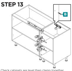
Check cabinets are level then clamp together. Pre-drill using 2mm drill bit and attach cabinets together.
