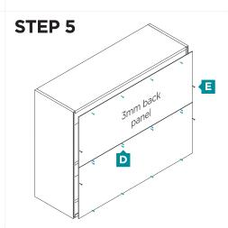
**note:** The white side of the back panel should face inside the cabinet.
