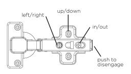
To align doors adjust marked screws.
