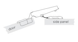
Clip the door onto the hinge plates.
