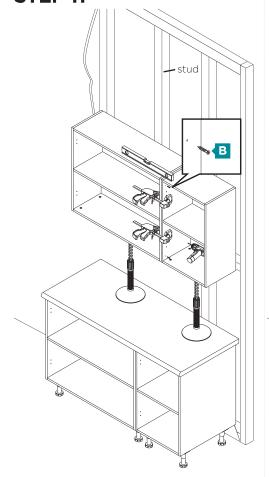
Check cabinets are level then clamp together. Pre-drill using 2mm drill bit and attach cabinets together.
