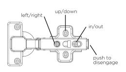
To align doors adjust marked screws.
